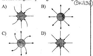
189. Which diagram best represents the electric field near a positively charged conducting sphere?
