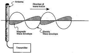
In what way did the electrons in the antenna produce the electromagnetic wave? (\$\int i\)
