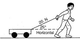
How much work does the child do in moving the wagon a horizontal distance of 4.0 meters?
