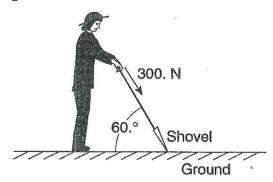
The component of the 300.-newton force that acts perpendicular to the ground is approximately (ie FAY)
