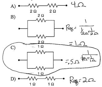
183. Three identical lamps are connected in parallel with each other. If the resistance of each lamp is X ohms, what is the equivalent resistance of this parallel combination?
