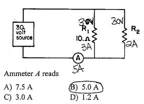
197. In the circuit diagram below, ammeter *A* measures the current supplied by the 10.-volt battery.
