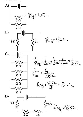
182. Which combination of resistors has the *smallest* equivalent resistance?
