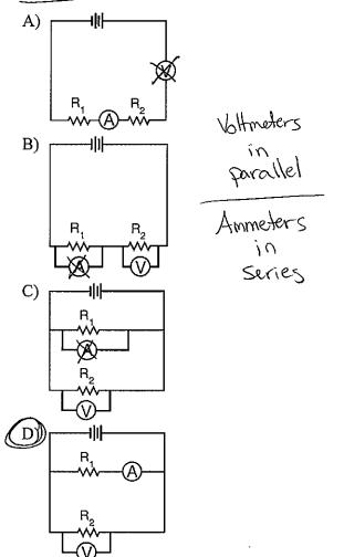
201. Which circuit diagram below correctly shows the connection of ammeter A and voltmeter V to measure the current through and potential difference across resistor R?
