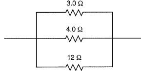
What is the equivalent resistance of this part of the circuit?
