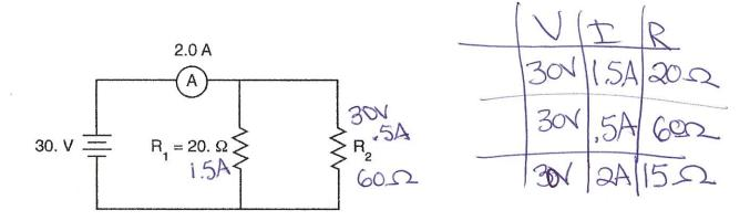
Calculate the resistance of resistor  $R_2$ . [Show all work, including the equation and substitution with units ]
